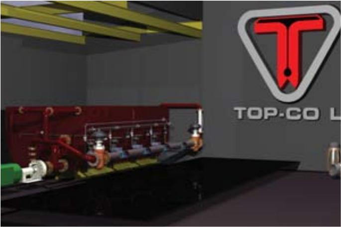
bilities to the company’s products and processes. Specifically, the facility will allow for the dynamic and rigorous testing of float equipment under divergent simulated downhole conditions including pressure, solid contents, heat and other variables. All test data will be electronically controlled and logged. This scientific study of tool performance under actual well conditions will enable Top-Co to verify product performance and provide empirical input for its continuous improvement program.
